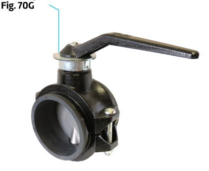
The Fig. 70G Butterfly Valve is designed for use with Gruvlok couplings, an ASC Engineered Solution, for fast and easy installation on grooved pipe. The valve body is fully rubber lined in EPDM or Nitrile material. A 316 Stainless Steel Disc is standard. The valve is supplied with a two position lockable handle.
